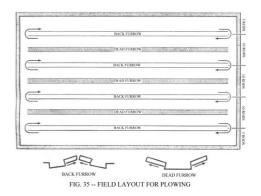
Throw a new back furrow in the same manner at the next back furrow line and plow around it until the unplowed portion between the lands equals that which has been plowed around the new back furrow. To reduce driving distance, plow around the unplowed portion between the two back furrows until it is completed to form a dead furrow. When plowing the dead furrow, set the plows shallow to prevent forming an objectionable trench the length of the field.
